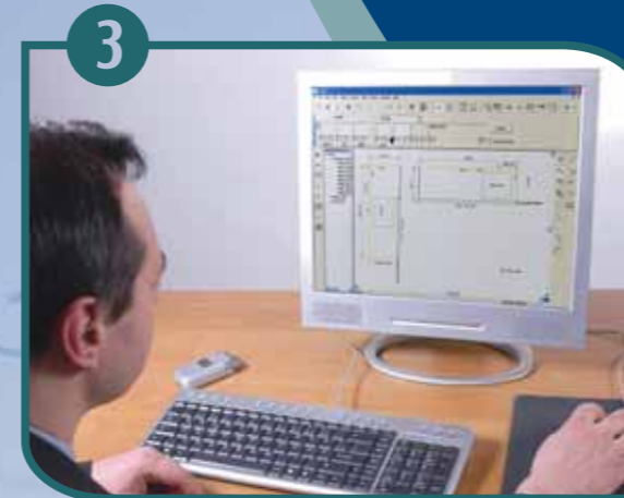
3 The electronic template received at the factory for production pre-processing, such as setting the seams and edge profiles, inserting sinks and stove cut-outs etc.
