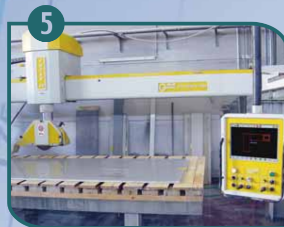
5 The electronic template is downloaded to the cutting machine. This can be: • Saw cutter • Water-Jet cutter • CNC
