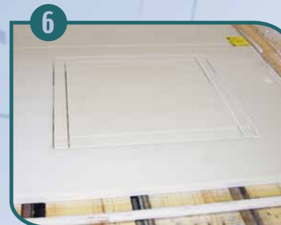
6 Countertop cut according to the electronic template.
